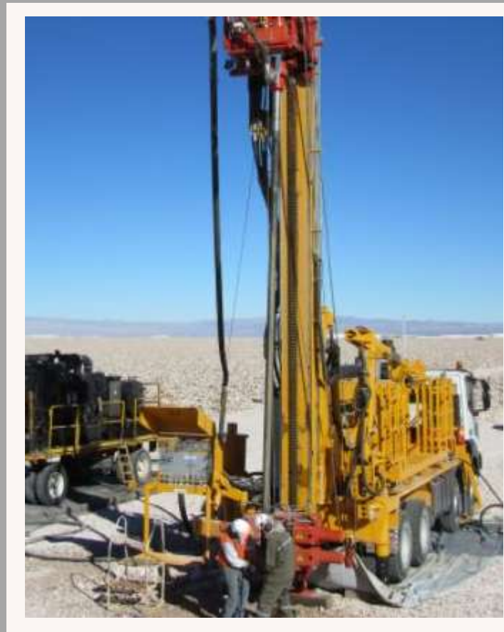
Reverse Circulation Drilling
